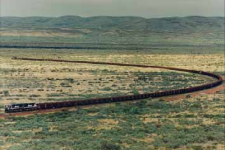
A typical 25,000 tonne train snakes its way to the coast. The BHP railway once operated the world's largest train, over 4 times the size of this one.
