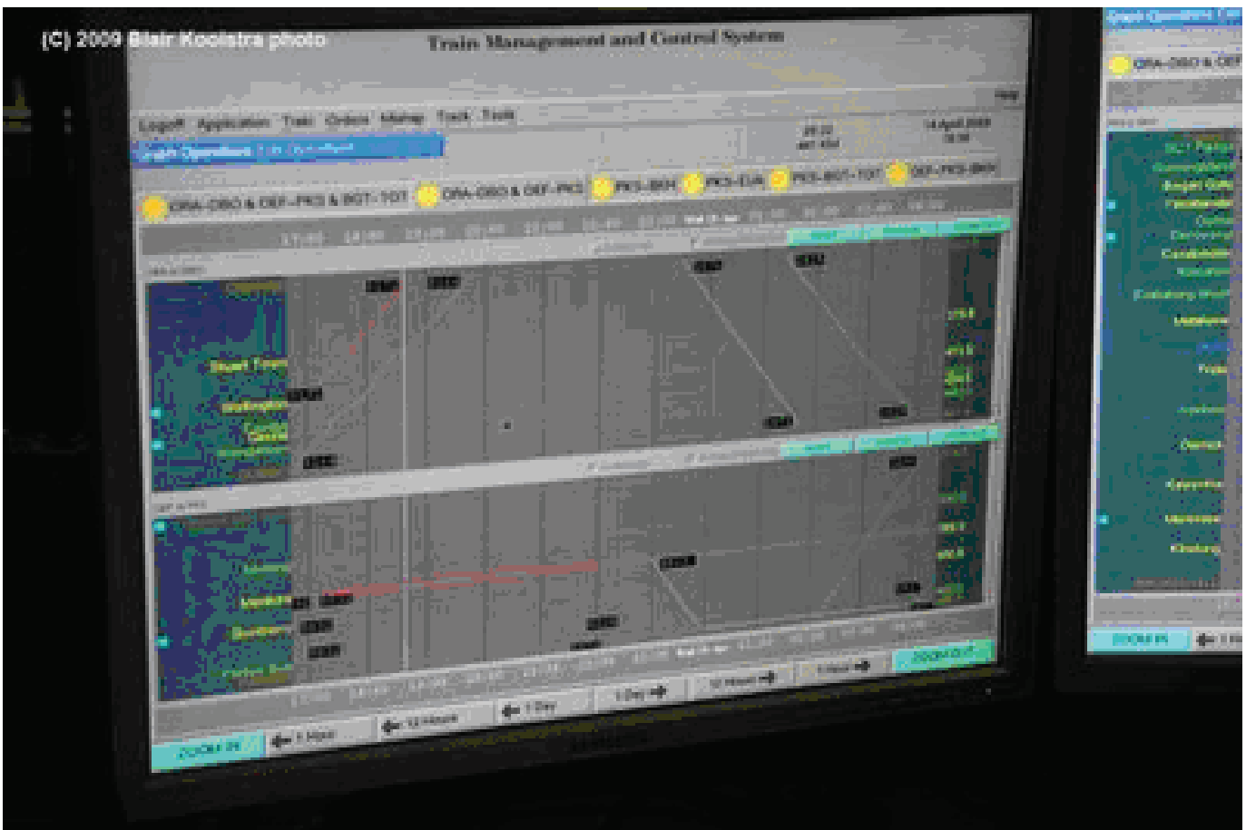
Overview screen for the train authority computer, automatically updates the location of trains via the GPS on locomotives and advances their location on the graph.
