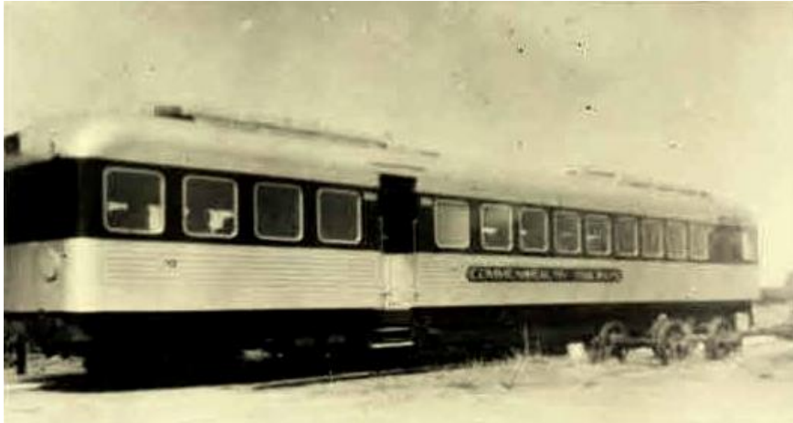
One of the new Gloucester 'NDH' class railcars taken at the no.2 end. (Photographer, Fred Davies, Image courtesy of the NT Library Service .)
