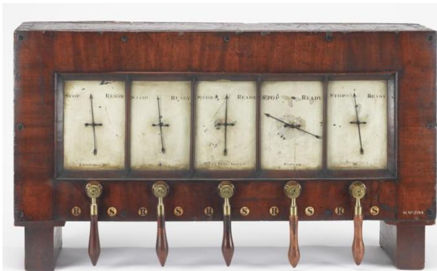
Blackwall Railway 5-needle Block Instruments (1840)
